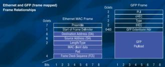
GFP Core Header: The four octets of the GFP Core Header consist of a 16-bit PDU Length Indicator field and a 16-bit Core Header Error Check (cHEC) field. This header al-
